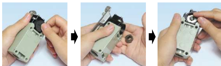
Loosen the cam holder with a coin or screw driver → Reverse the cam → Reverse the position of the cam and reinstall
