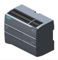
SIMATIC S7-1200, CPU 1215C, compact CPU, DC/DC/relay, 2 PROFINET ports, onboard I/O: 14 DI 24 V DC; 10 DO relay 2 A, 2 AI 0-10 V DC, 2 AO 0-20 mA DC, power supply: DC 20.4-28.8 V DC, program/data memory 200 KB
