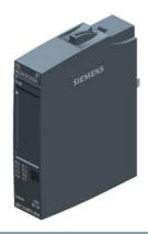
SIMATIC ET 200SP, Digital output module, DQ 8x 24V DC/0,5A Standard, Source output (PNP,P-switching) Packing unit: 1 piece, fits to BU-type A0, Colour Code CC02, substitute value output, module diagnostics for: short-circuit to L+ and ground, wire break, supply voltage
