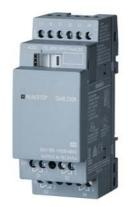
LOGO! DM8 230R expansion module, PS/I/O: 230V/230V/relay, 2 MW, 4 DI/4 DO for LOGO! 8  $\,$
