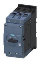
Circuit breaker size S3 for motor protection, CLASS 10 A-release 75...93 A N-release 1300 A screw terminal Standard switching capacity
