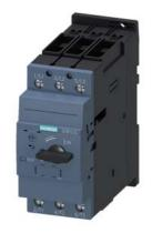
Circuit breaker size S2 for motor protection, CLASS 10 A-release 32...40 A N-release 585 A screw terminal Standard switching capacity
