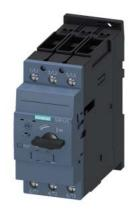
Circuit breaker size S2 for motor protection, CLASS 10 A-release 28...36 A N-release 520 A screw terminal Standard switching capacity
