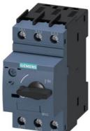
Circuit breaker size S0 for motor protection, CLASS 10 A-release 23...28 A N-release 364 A screw terminal Standard switching capacity
