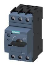
Circuit breaker size S0 for motor protection, CLASS 10 A-release 13...20 A N-release 260 A screw terminal Standard switching capacity
