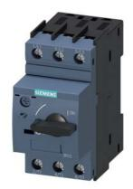
Circuit breaker size S00 for motor protection, CLASS 10 A-release 0.7...1 A N-release 13 A screw terminal Standard switching capacity
