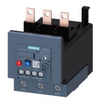
Overload relay 57...75 A Thermal For motor protection Size S3, Class 10 Contactor mounting Main circuit: Screw Auxiliary circuit: Screw Manual-Automatic-Reset
