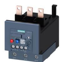
Overload relay 36...50 A Thermal For motor protection Size S3, Class 10 Contactor mounting Main circuit: Screw Auxiliary circuit: Screw Manual-Automatic-Reset
