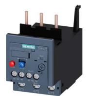
Overload relay 70...80 A Thermal For motor protection Size S2, Class 10A Contactor mounting Main circuit: Screw Auxiliary circuit: Screw Manual-Automatic-Reset
