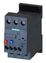
Overload relay 30...36 A Thermal For motor protection Size S0, Class 10 Standalone installation Main circuit: Screw Auxiliary circuit: Screw Manual-Automatic-Reset
