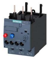
Overload relay 30...36 A Thermal For motor protection Size S0, Class 10 Contactor mounting Main circuit: Screw Auxiliary circuit: Screw Manual-Automatic-Reset
