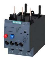
Overload relay 14...20 A Thermal For motor protection Size S0, Class 10 Contactor mounting Main circuit: Screw Auxiliary circuit: Screw Manual-Automatic-Reset
