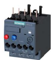
Overload relay 3.5...5.0 A Thermal For motor protection Size S00, Class 10 Contactor mounting Main circuit: Screw Auxiliary circuit: Screw Manual-Automatic-Reset
