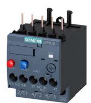
Overload relay 1.4...2.0 A Thermal For motor protection Size S00, Class 10 Contactor mounting Main circuit: Screw Auxiliary circuit: Screw Manual-Automatic-Reset
