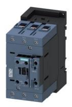
power contactor, AC-3e/AC-3, 95 A, 45 kW / 400 V, 3-pole, 230 V AC, 50/60 Hz, auxiliary contacts: 1 NO + 1 NC, screw terminal, size: S3  $\,$
