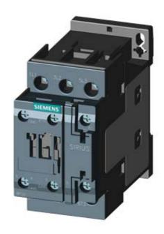
CONTACTOR, AC-3, 5.5KW/400V, 1NO+1NC, AC110V 50/60HZ, 3-POLE, SZ SO SCREW TERMINAL
