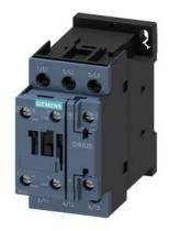
power contactor, AC-3e/AC-3, 9 A, 4 kW / 400 V, 3-pole, 230 V AC, 50/60 Hz, auxiliary contacts: 1 NO + 1 NC, screw terminal, size: S0
