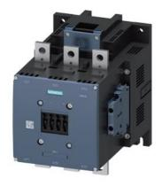
power contactor, AC-3e/AC-3 500 A, 250 kW / 400 V AC (50-60 Hz) / DC Uc: 440-480 V 3-pole, auxiliary contacts 2 NO + 2 NC drive: conventional main circuit: busbar control and auxiliary circuit: screw terminal
