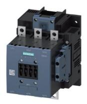
power contactor, AC-3e/AC-3 150 A, 75 kW / 400 V AC (50-60 Hz) / DC Uc: 440-480 V 3-pole, auxiliary contacts 2 NO + 2 NC drive: conventional main circuit: busbar control and auxiliary circuit: screw terminal
