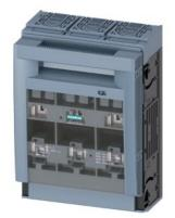
SENTRON, Fuse switch disconnector 3NP1, 3-pole, NH2, 400 A, for assembly and installation on mounting plate, flat terminal, cover level 70  $\,\mathrm{mm}$
