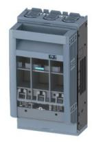
SENTRON, Fuse switch disconnector 3NP1, 3-pole, NH00, 160 A, for assembly and installation on mounting plate, flat terminal, Cover level 45 mm
