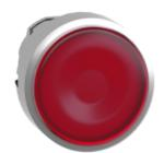
Head for illuminated push button, Harmony XB4, metal, red flush, 22mm, universal LED, push-push, unmarked
