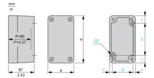
(2)  $2 \times \emptyset$  5.6 mm/4.94 in. holes, depth 12 mm/0.47 in. Usable depth
