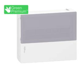
Enclosure, Resi9 MP, surface mounting, 1 row of 12 modules, IP40, translucid door, 1 earth + 1 neutral terminal blocks
