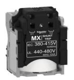
MX shunt release, ComPacT NSX, rated voltage 380/415 VAC 50/60 Hz, 440/480 VAC 60 Hz, screwless spring terminal connections
