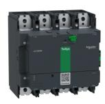
High power contactor, TeSys Giga 800,4P(4NO), AC-1 <=440V 1050A, standard version, 48-130V AC/DC wide band coil
