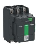
High power contactor, TeSys Giga, 3 pole (3NO), AC-3 <=440V 500A, standard version, 48...130V wide band AC/DC coil
