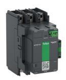
High power contactor, TeSys Giga, 3 pole (3NO), AC-3 <=440V 150A, standard version, 100...250V wide band AC/DC coil
