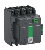
High power contactor, TeSys Giga, 4 pole (4NO), AC-1 <=440V 275A, standard version, 48...130V wide band AC/DC coil
