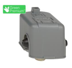
Pressure sensors XM, pressure switch FSG 4.6 bar, adjustable scale 2 thresholds, 2NC
