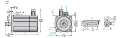
a: Power supply for servo motor brake Power supply for servo motor encoder Shaft end, keyed slot (optional) For screw M6 x 21 mm/M6 x 0.83 in. b: (1) (2)
