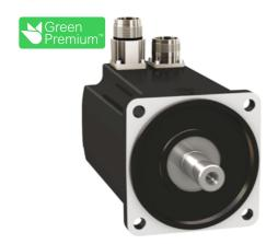
servo motor BMH, Lexium 32, 8.4Nm, 6000rpm, keyed shaft, without brake, IP54, 16bit encoder, straight
