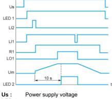
LED 1: Green LED LI2, LI1 : Logic inputs R1 : Relay output LO1 : Logic output Um : Motor voltage
