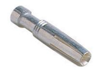
Female crimp contact, CC series, 16 A, turned silver plated, wire cross section 1,5 mm<sup>2</sup>, AWG 16
