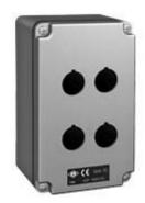
Box for control devices and signals, AC series, without cable entry, 4 holes for unit  $\emptyset$  22 mm, external dimensions 92x152x86 mm
