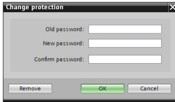
Figure 11-6 Removing know-how protection for blocks
