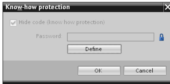
Figure 11-5 Setting up block know-how protection (2)
