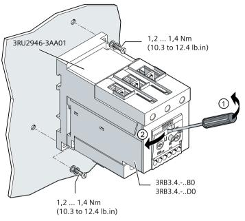
Mounting the 3RB3.4 electronic overload relay, stand-alone installation (screw mounting)
