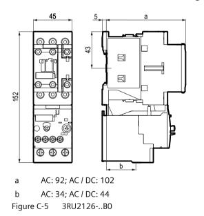
C.2 Dimension drawings for 3RU21 thermal overload relays
