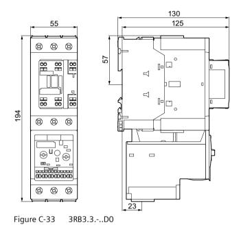
3RB3.3.-..D0 (S2, spring-loaded connection, mounting on stand-alone assembly support)
