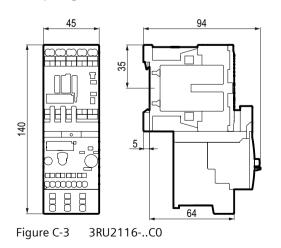
C.2 Dimension drawings for 3RU21 thermal overload relays
