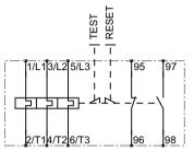
Figure 13-6 3RB20, S6 electronic overload relay
