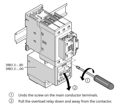
Disassembly of the 3RB3.3 electronic overload relay screw-type connection system
