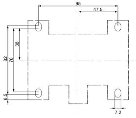
Figure C-20 3RB2.5-..W / 3RB2.5-..X drilling plans
