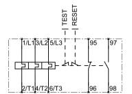
Figure 13-13 3RB30 electronic overload relay, S2
