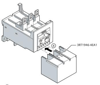
(4) Slide the terminal cover for cable lug connection and busbar connection into the guide tabs on the overload relay.
