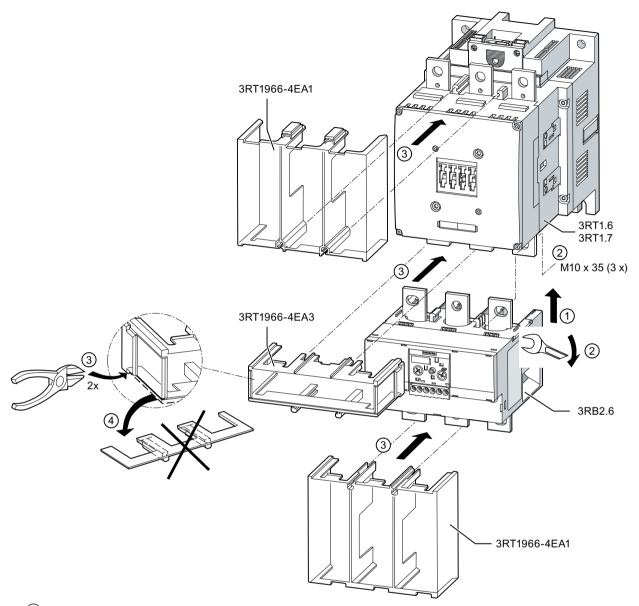
Mounting the 3RB2.6 electronic overload relay (busbar connection)
