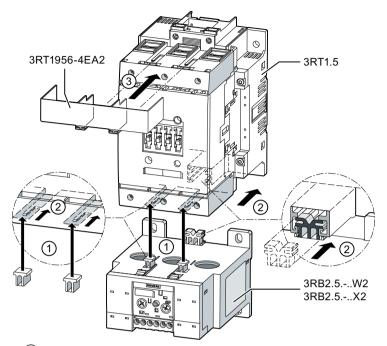
Mounting the 3RB2.5 electronic overload relay (connection with box terminal block and through-hole technology)
