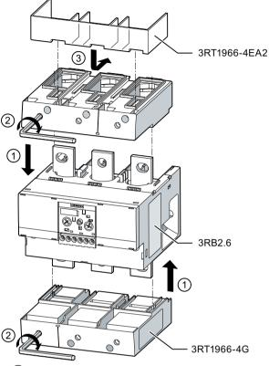
Mounting the 3RB2 electronic overload relay (connection with box terminal block)
