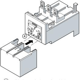
(4) Slide the terminal cover for cable lug connection and busbar connection into the guide tabs on the overload relay.
