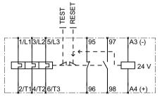
Figure 13-18 3RB31 electronic overload relay, S2
