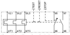
Figure 13-3 Thermal overload relay, SO
