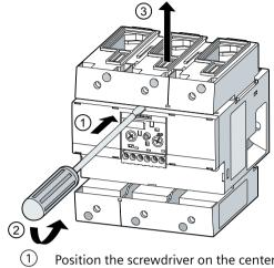
Disassembling the 3RB2 electronic overload relay (connection with box terminal block)
