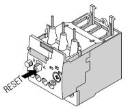
Figure 10-3 Resetting following device test
