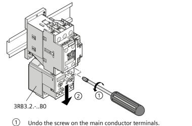
Disassembly of the 3RB3.2 electronic overload relay screw-type connection system
