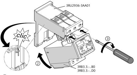
$\begin{pmatrix} 1 \\ 2 \end{pmatrix}$  Guide the overload relay into the terminal support from below with a swivel movement
