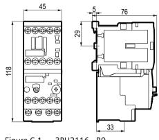
3RU2116-..B0 (S00, screw connection, contactor mounting)
