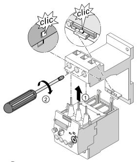
① Guide the overload relay into the terminal support from below.
