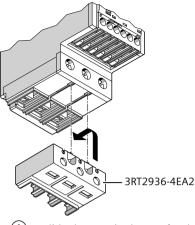
(1) Slide the terminal cover for the box terminal block into the openings provided on the box terminal block of the overload relay.
