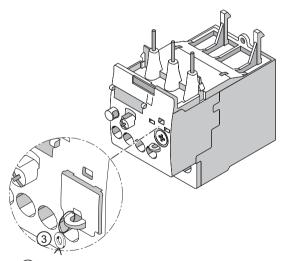
③ Seal the cover to secure it against unauthorized removal.
