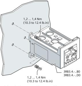
Mounting the 3RB3.4 electronic overload relay, stand-alone installation (through-hole technology)
