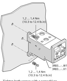
Mounting the 3RB3.3 electronic overload relay, stand-alone installation (through-hole technology)
