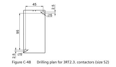
C.5 Drilling diagram for 3RT contactors
