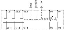
Figure 13-4 Thermal overload relay, S2
