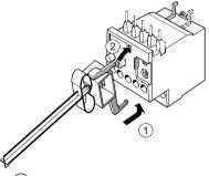
Attach the hook on the release slide to the designated opening on the overload relay.
