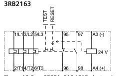
Figure 13-9 3RB21, S10 / S12 electronic overload relay
