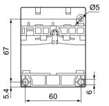
Figure C-42 3RB3.4.-..W. - drilling diagram
