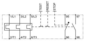
Figure 13-2 Thermal overload relay, spring-loaded connection system, S00
