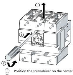
Disassembly of the 3RB2.6 electronic overload relay (connection with box terminal block)
