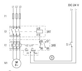
1 Electrical remote RESET (3RB31 only) Figure 13-23 3RB3.3.-...
