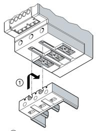
(1) Slide the terminal cover for the box terminal block into the openings provided on the box terminal block of the overload relay.
