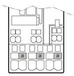
Figure 8-2 Main conductor terminals on the contactor (a) (S0)
