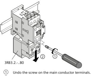
2 Pull the overload relay down and away from the contactor.
