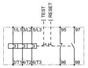
Figure 13-12 3RB30 electronic overload relay, S0
