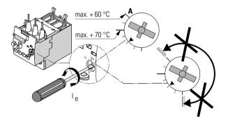
Figure 10-1 Setting the current I<sub>e</sub>
