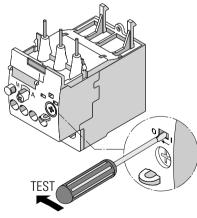
Figure 10-2 Executing a device test
