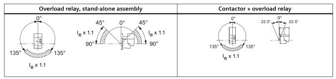
The set value is 1.1 times the motor current for a mounting position in the hatched area.
