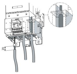
Observe a stripped length of 20 mm when connecting.
