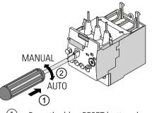
1 Press the blue RESET button down with a screwdriver.
