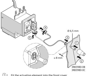
Mounting a mechanical remote RESET to a 3RB3.3 electronic overload relay.
