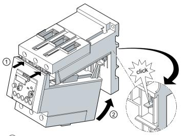
Guide the overload relay into the terminal support from below with a swivel movement.
