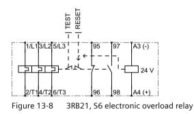
13.5 Internal circuit diagrams 3RB30
