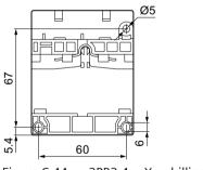
Figure C-44 3RB3.4.-..X. - drilling diagram
