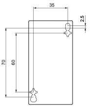
Figure C-47 Drilling plan for 3RT2.2. contactors (size S0)
