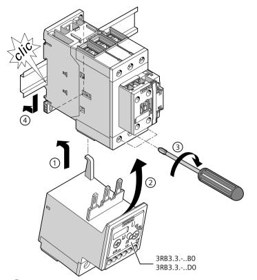
Mounting the 3RB3.3 electronic overload relay, screw-type connection system
