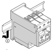
(4) Position the terminal support with mounted overload relay on the top edge of the DIN rail and press it down until it snaps onto the bottom edge of the DIN rail.
