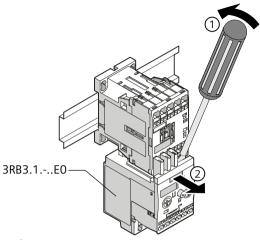
Disassembly of the 3RB3.1 electronic overload relay spring-loaded connection system
