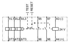
Figure 13-19 3RB31 electronic overload relay, S3
