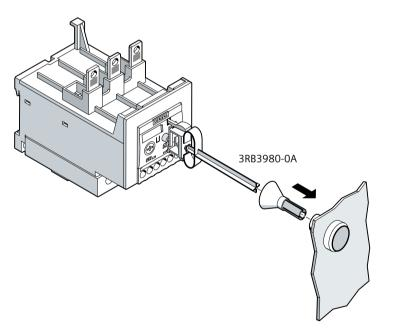
Mounting a mechanical remote RESET to a 3RB3.4 electronic overload relay.
