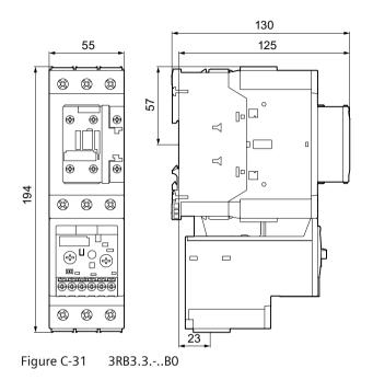
3RB3.3.-..B0 (S2, screw connection, mounting on stand-alone assembly support)
