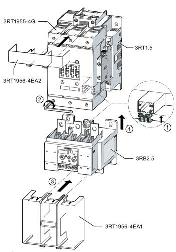
Mounting the 3RB2.5 electronic overload relay (connection with box terminal block)
