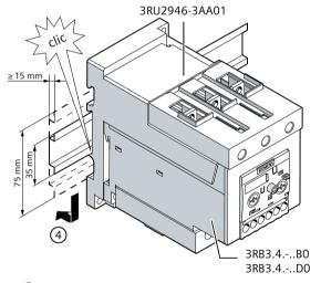
(4) Position the terminal support with mounted overload relay on the top edge of the DIN rail and press it down until it snaps onto the bottom edge of the DIN rail.
