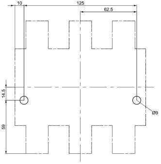
Figure C-22 3RB2.6 drilling plan
