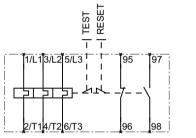
Figure 13-14 3RB30 electronic overload relay, S3
