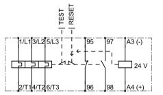
Figure 13-17 3RB31 electronic overload relay, S0
