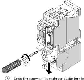
Undo the screw on the main conductor terminals.
