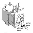
① Using a screwdriver, slide the switch to the required position.
