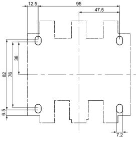
Figure C-18 3RB2.5 drilling plan
