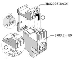
(1)Insert the contacts into the central opening of the main conductor terminals on the terminal support, with the contacts flush to the right.
