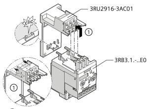
(1) Insert the contacts into the central opening of the main conductor terminals on the terminal support.
