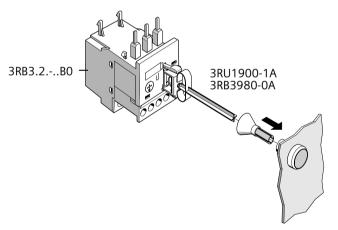
Mounting a mechanical remote RESET to a 3RB3.2 electronic overload relay.
