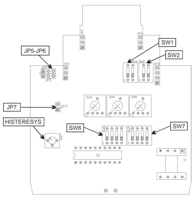
Internal jumper setting for <u>standard</u> <u>inputs</u>:
