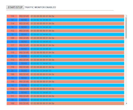
The first column is the delay in milliseconds from the last packet, the second column is the direction of the packet (received from or transmitted to), the last column is the contents of the packet in hexadecimal format. Only the serial ModBUS stream is displayed.
