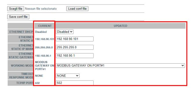
The first column represents the name of the parameter, the second column "current" is the current value of the parameter. The last column "updated" is used to modify the current configuration.
