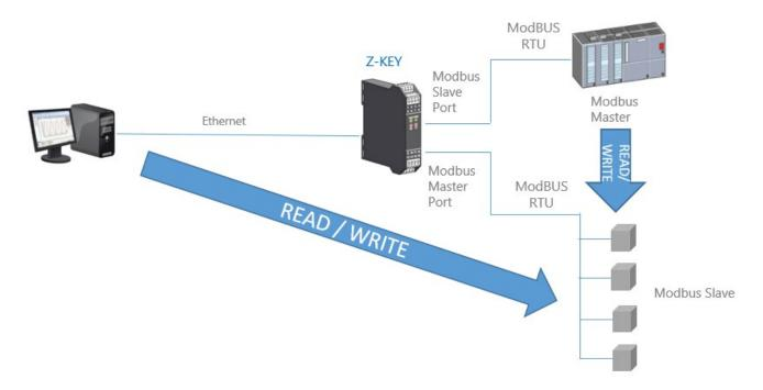
This function is possible because the Seneca Gateway uses an internal memory shared between the serial ports and the Ethernet port, where the data acquired from the serial Modbus Slave network are saved.
