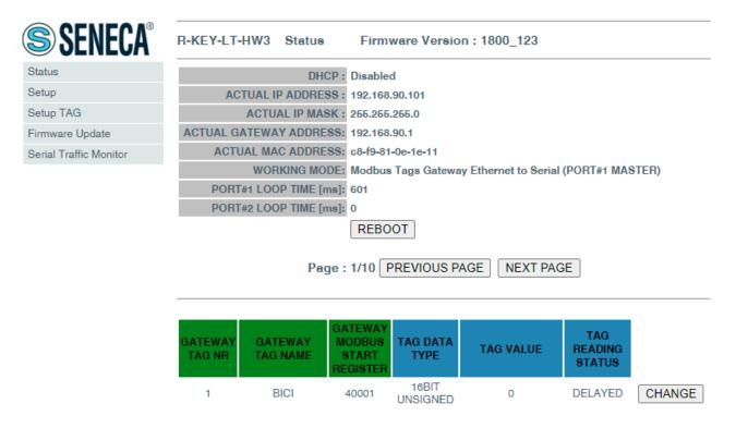
Tag information includes: The name of the TAG, the Modbus address of the TAG Gateway, the value of the Tag and the status of the TAG:
