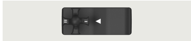
Fig. 2: Star handle for adjustment of latching force
