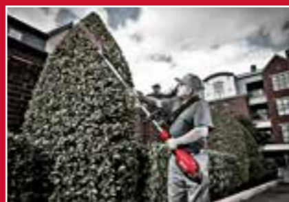
Articulating head offers 12 positions from 0° to 270° for the most comfortable user sculpting angles and easy trimming the top of tall hedges
