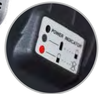
●Power indicator ● Active / standby ☀ Power is on ☀ Power is low ☀ Overcurrent protection
