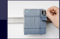
Removable high(er) density terminal blocks with push-in wiring for ease of use → non-contact pre-wiring position.
