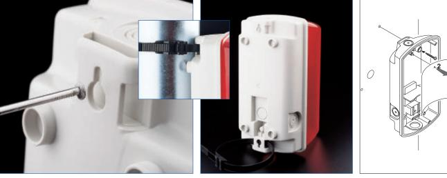
MIZAR Series light-fittings are fitted with a slot on the rear of the base for or scaffolding using one or two cable ties. For permanent installation, the hooking onto a nail, screw or hook, or for fastening to poles, pipes, bars fixtures can be wall or ceiling mounted using screw anchors.
