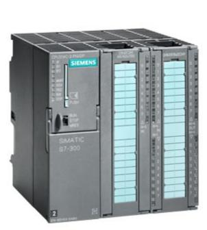
SIMATIC S7-300, CPU 314C-2PN/DP COMPACT CPU WITH 192 KBYTE WORKING MEMORY, 24 DI/16 DO, 4AI, 2AO, 1 PT100, 4 FAST COUNTERS (60 KHZ), 1. INTERFACE MPI/DP 12MBIT/S, 2. INTERFACE ETHERNET PROFINET, WITH 2 PORT SWITCH, INTEGRATED 24V DC POWER SUPPLY, FRONT CONNECTOR (2 X 40PIN) AND MICRO MEMORY CARD REQUIRED
