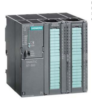
SIMATIC S7-300, CPU 314C-2 DP COMPACT CPU WITH MPI, 24 DI/16 DO, 4AI, 2AO, 1 PT100, 4 FAST COUNTERS (60 KHZ), INTEGRATED DP INTERFACE, INTEGRATED 24V DC POWER SUPPLY, 192 KBYTE WORKING MEMORY, FRONT CONNECTOR (2 X 40PIN) AND MICRO MEMORY CARD REQUIRED
